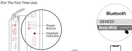
① Long press the power button for 3S, and the indicator light flashes in red or blue alternately, entering Bluetooth pairing mode. (Sound: Bluetooth Mode)
