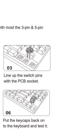
Gently press the switch PCB and integrate it closely. into place.
